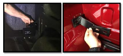
B) If the bed has a D-Rings in the front you will use the supplied bolt/washer/nut, mount plate and spacers to sandwich the D-Ring between the mount plate and the bracket.
